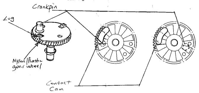
Alternatively the winscreen wiper box can be rotated through 180°. See diagram below:-
