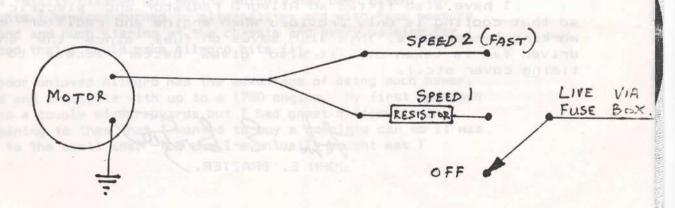
An alternative would be to fit a rheostat control from another car and have a variable speed fan.
