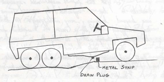
Anybody about to build might find it better to locate a tank in one of the rear subframes. this would obviously produce a more constant ground clearance.
